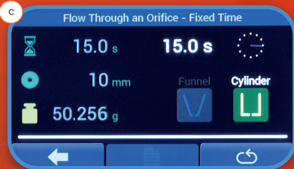
A: Angle of Repose B: Bulk Density C: Flow Through an Orifice via Cylinder – Fixed Time Density D: Flow Through an Orifice via Funnel – Fixed Mass
